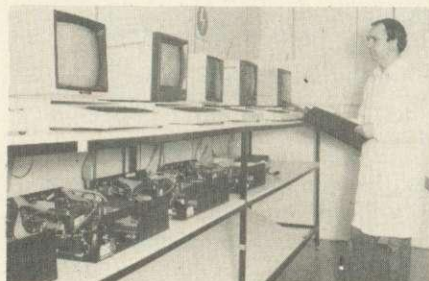
Winchester Disc Drives are put through a 24 hour intensive test programme prior to despatch to customers around the world.
